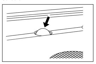
The solar sensor, located in the defrost grille, middle of the instrument panel, monitors the solar radiation. Do not cover the solar sensor or the system will not work properly.
